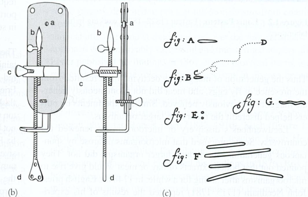
**Figure 1.1** **Antony van Leeuwenhoek.** Leeuwenhoek (1632–1723) and his microscopes. (a) Leeuwenhoek holding a microscope. (b) A drawing of one of the microscopes showing the lens, *a*; mounting pin, *b*; and focusing screws, *c* and *d*. (c) Leeuwenhoek’s drawings of bacteria from the human mouth.
